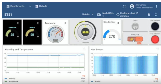
Fig. 4 Graphs and data for temperature, Humidity and Gas Sensors in WSN Monitoring Application (Open Source IoT platform: Thingsboard.io)
